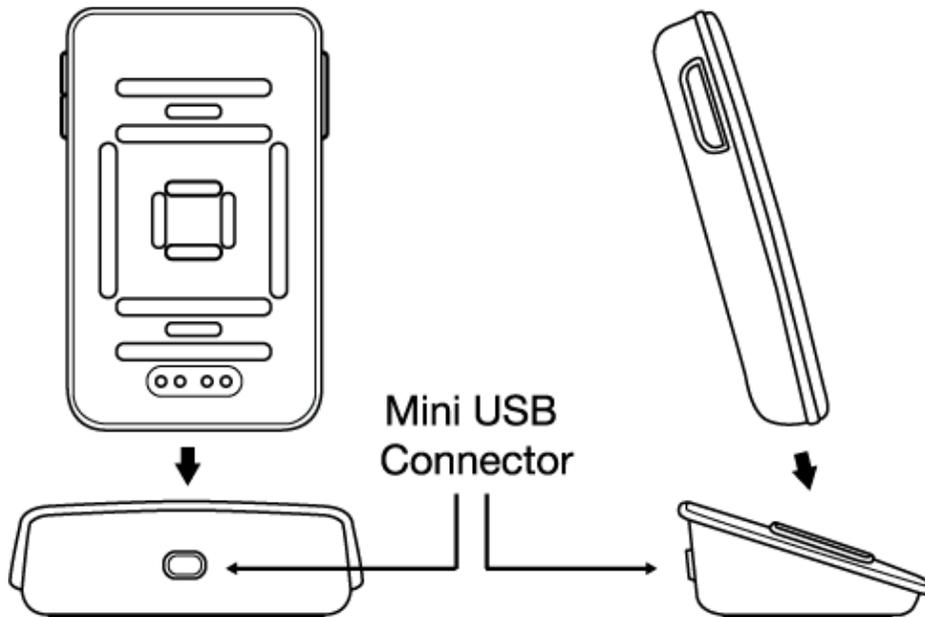
To charge it, place your Aim inside the cradle, to ensure the four pins on the back of Aim are making contact with those in the cradle. Plug in the Mini USB cable into the Mini USB connector on the charging cradle. Plug in the other end of the cable (USB) into the USB port on your computer (or similar device). The USB must be powered from a UL 60950-1 listed device.
